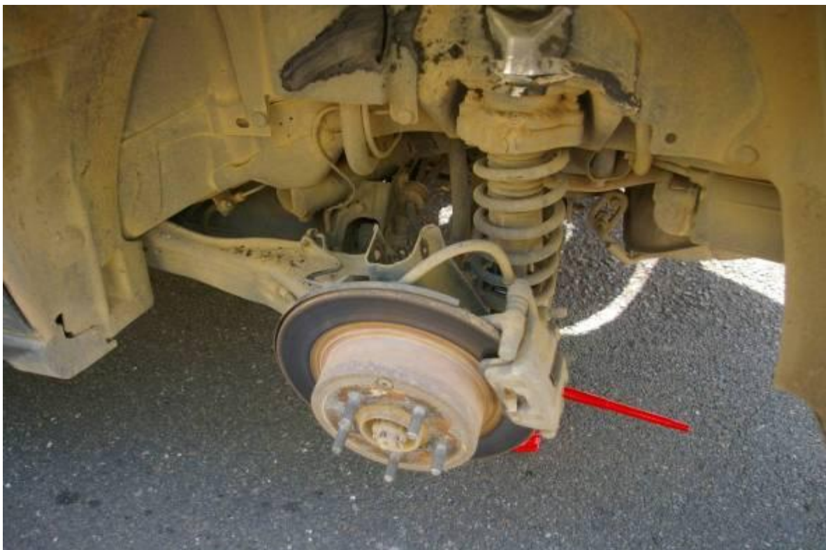
Busted suspension With supporting bar removed
